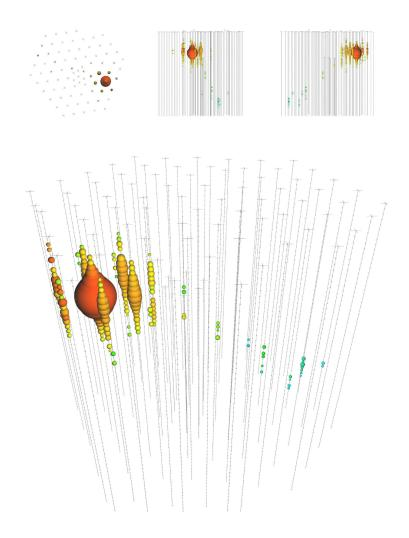
In the graphical rendering, each DOM is shown by a white dot. Colored spheres show sensors that have detected light. The size scales with the amount of recorded light and the color indicates arrival time (red first, green last, so in our case the neutrinos clearly traveled from the left to the right).
